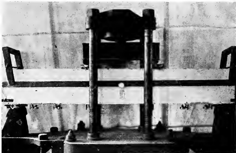
(a) Showing Instruments for Measuring Center Deflection and Slip of Bar at Intermediate Points.
